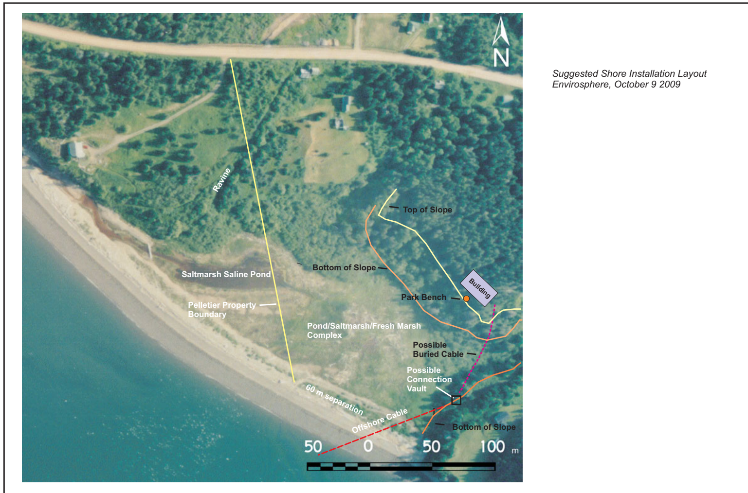
Figure 2.0-2: Aerial view of the study area showing the proposed shore installation layout for the building and the offshore cable.
