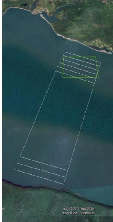
Figure 2: Transects completed for the fish hydroacoustic surveys. The green square indicates the FORCE test site whereas the white lines highlight the transects completed through the test site and control site (bottom of image) near Cape Split.
