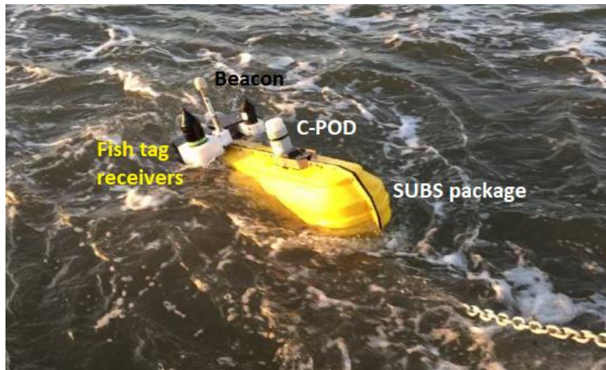
Figure 3: Recently deployed SUBS package containing two fish tag receivers, a beacon from MetOcean Telematics, and C-POD.
