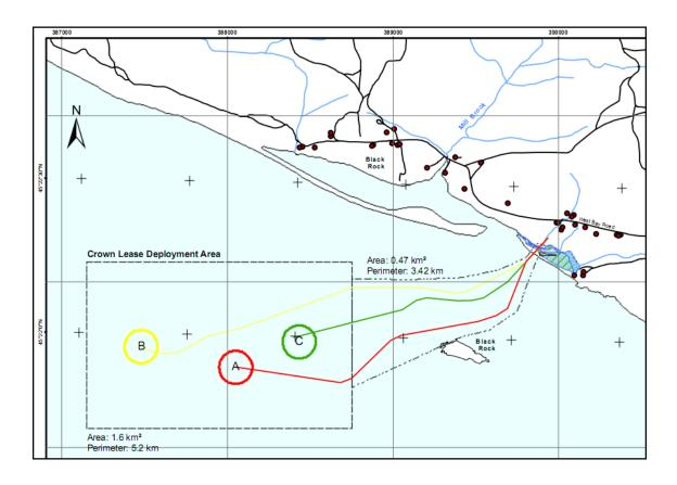
**Figure 6.** Map of the northern side of the Minas Passage, showing the FORCE crown lease deployment area (rectangle) and the locations of turbine berth areas A, B, and C and associated cable routes (Source: AECOM, 2009).
