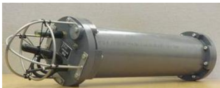
Figure 7. Autonomous Multichannel Acoustic Recorder (AMAR; JASCO Applied Sciences).
