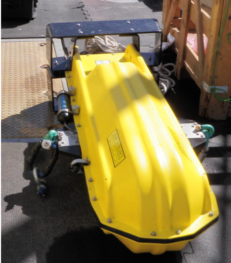
Figure 14. Streamlined float showing two of three hydrophones. Foreground: M8E hydrophone (small black cylinder underneath a gray clamp at the top left of the streamlined float). Background: M56 hydrophone (blue and black torpedo-shaped hydrophone). The M56 hydrophone has six hydrophone elements spaced throughout the volume. Similar to towed arrays, the intent of the M56 was to reduce flow noise by summing the elements to amplify external sound waves and cancel uncorrelated local flow noise.
