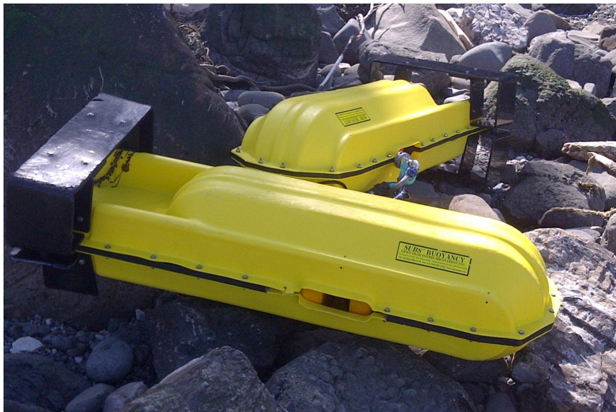
Figure 15. Streamlined floats at Scot's Bay, NS, 28 Mar 2012. The black HDPE frame of the streamlined float in the foreground had failed.
