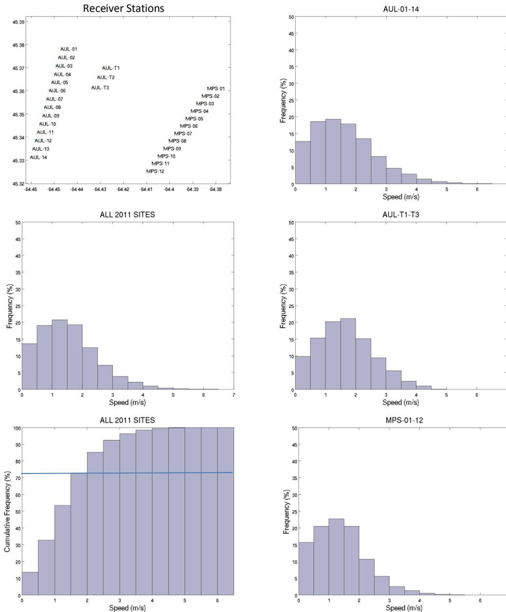
**Figure 2.11.** Top left: receiver stations. Frequency distributions of average water column current speed (m/s) over a 2 month period, for all sites combined (left, middle) and for each of the three receiver lines (AUL, AUL-T and MPS) (right side, top to bottom). The bottom left panel features cumulative frequency for average current speed and shows that during about 30% of the time, average water column current speeds are greater than 2 m/s.
