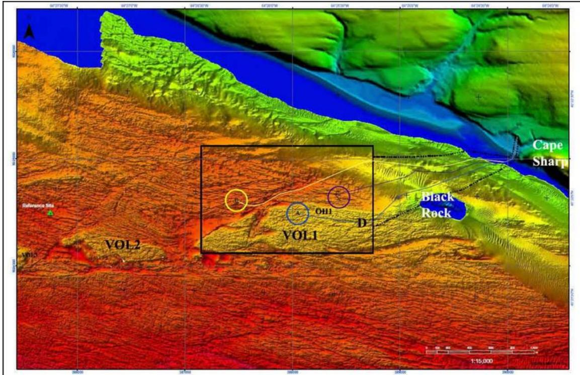
**Figure 2.4.** Multibeam bathymetric map of the FORCE test area and surrounds in Minas Passage, Bay of Fundy, showing volcanic platforms (VOL), gravel waves, troughs, and various bedforms. Black Rock is located east of the FORCE site. Source: GSC (in Fader, 2011).
