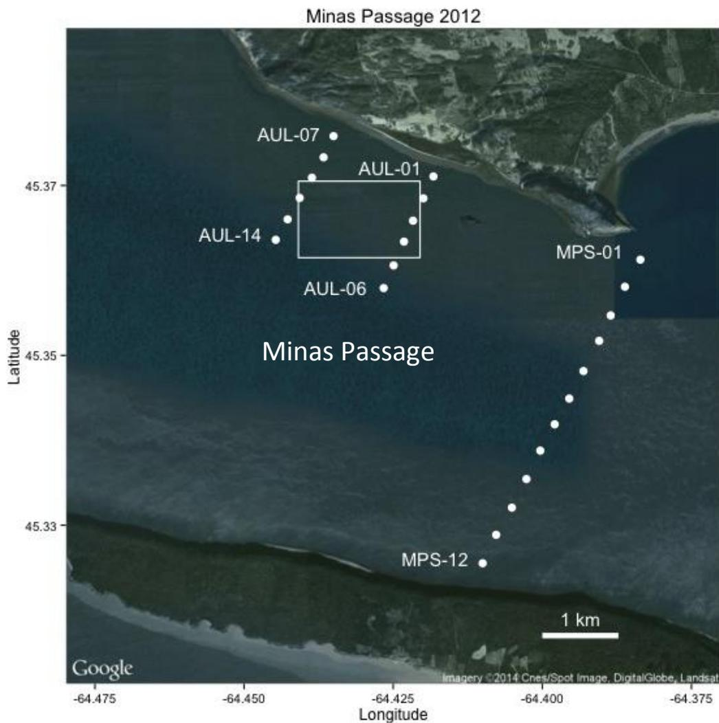
**Figure 2.7.** Positions of bottom moored VEMCO VR2w acoustic receiver stations deployed in Minas Passage, NS during 2012-2013. The shaded rectangle indicates the area of the FORCE demonstration site. Points AUL-01 to AUL-12 are station positions of the two Acadia University receiver lines, and MPS-01 to MPS-12 are station positions of the OTN-MPS line.
