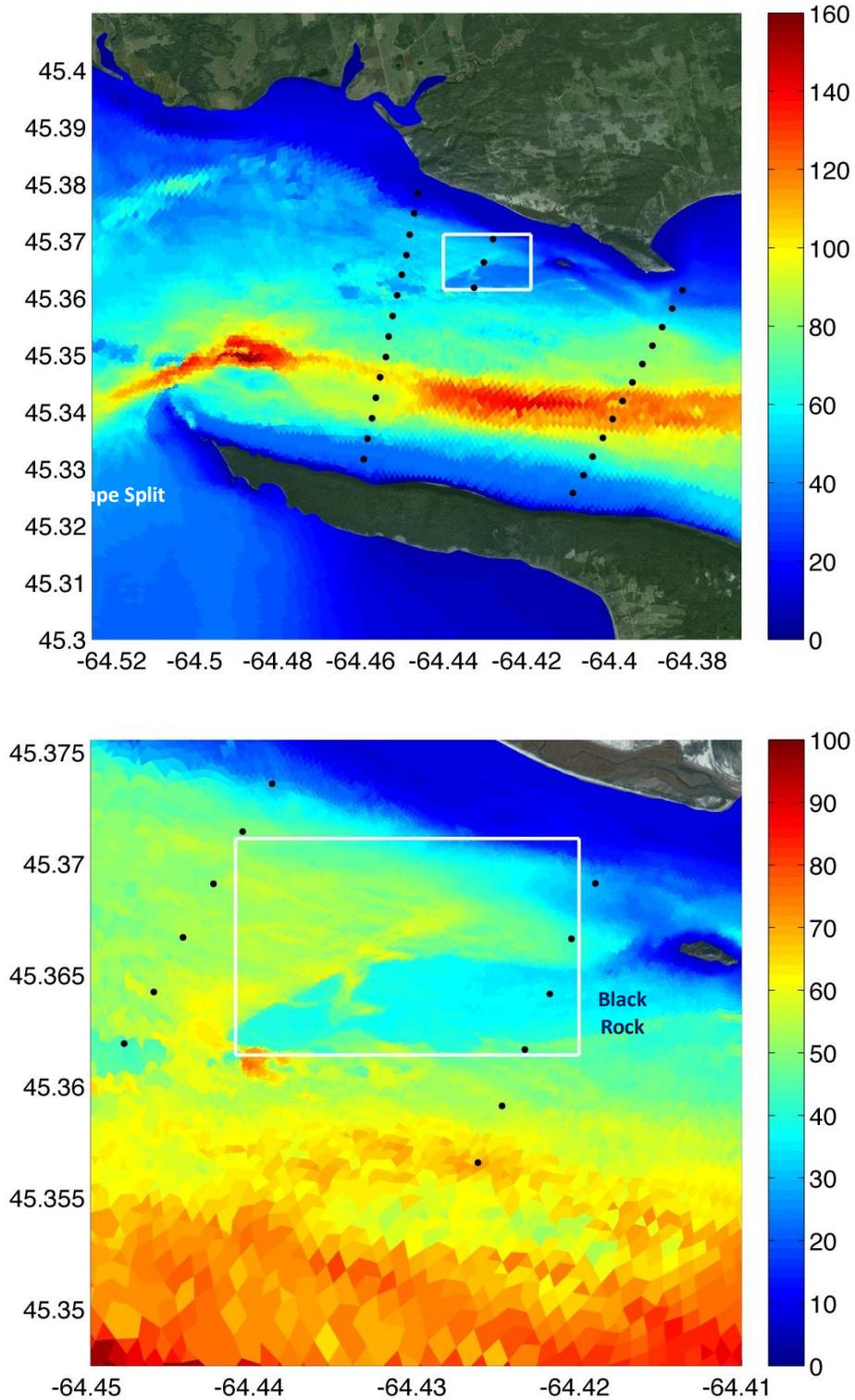
**Figure 2.1.** Mean water depths (m) in Minas Passage (top) and within and near the FORCE Crown Lease area (bottom). Locations of moored VEMCO receivers are indicated with the black dots and the white box is the FORCE lease area. Note the locations of Cape Split and Black Rock.
