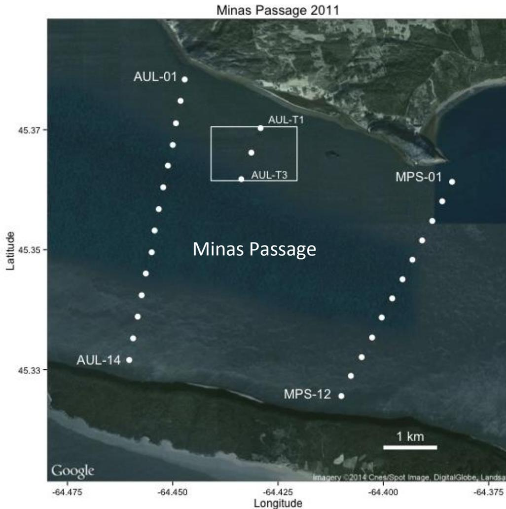
**Figure 2.6.** Positions of bottom moored VEMCO VR2w acoustic receiver stations deployed in Minas Passage, NS during 2011. The shaded rectangle indicates the area of the FORCE demonstration site. Dot points indicate the station positions of the Acadia University Line (AUL-01 to AUL-14), the FORCE Line (AUL-T1 to AUL-T3), and the OTN's MPS Line (MPS-01 to MPS-12).
