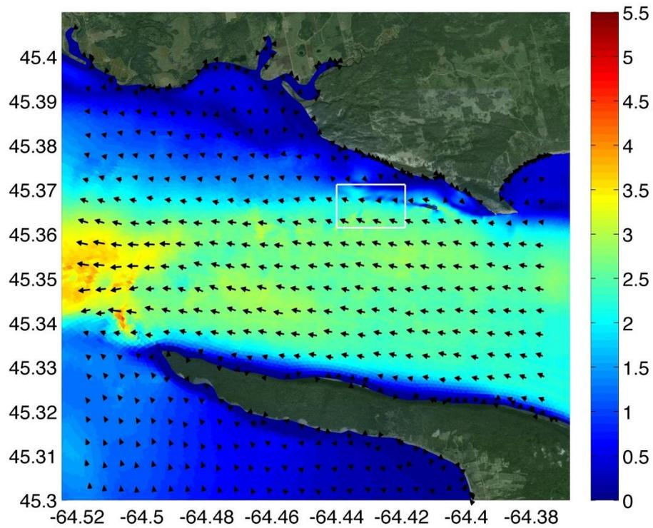
**Figure 2.2.** Predicted flow speeds (m/s) and direction in the Minas Passage during a typical flood tide (top) and a typical ebb tide (bottom). The arrows indicate the direction of the flow at the given location. The white box is the FORCE lease area.
