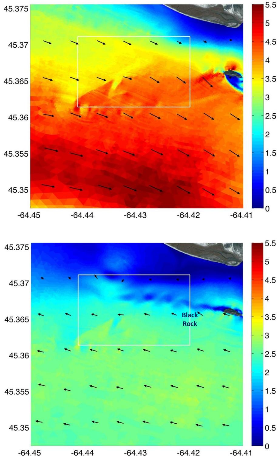
**Figure 2.3.** Predicted flow speeds (m/s) and direction in and near the FORCE Crown Lease area during a typical flood tide (top) and a typical ebb tide (bottom). The arrows indicate the direction of the flow at the given location. The white box is the FORCE lease area.
