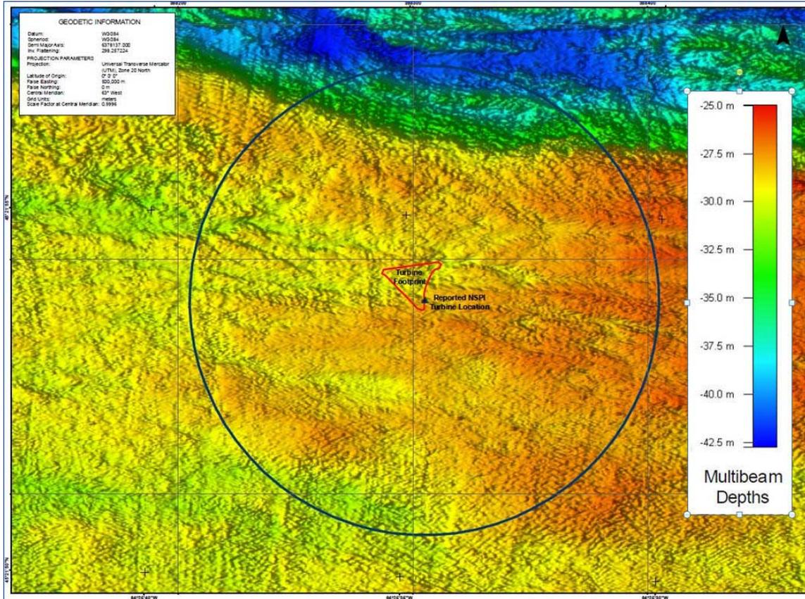
**Figure 6** A multibeam bathymetric shaded relief map of the NSPI/OH1 site showing the location of the device (red triangle) relative to detailed bathymetry. The multibeam data was collected by Seaforth Geosurveys and is presented at 0.5 m resolution. The CHS reported location for the device is also shown as a small black triangle. The circle is 200 m in diameter centered on the officially reported position.
