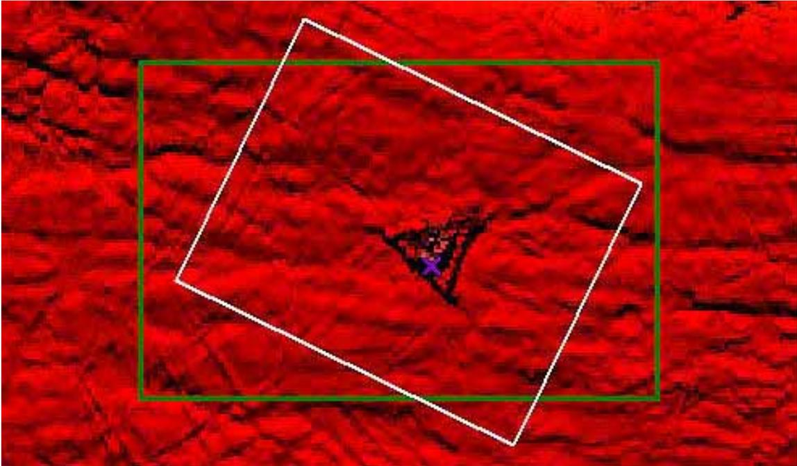
**Figure 5** A multibeam bathymetric map of the seabed during the deployed phase of NSPI/OH1 by Seaforth Geosurveys Inc. showing the shape of the gravity platform and the surrounding topography of the seabed. This information provided the exact georeferenced location of the device. X marks the position of the coordinates of the device provided by the Canadian Hydrographic Service. North is to the top of the image and the device is 21 by 25 m in size.
