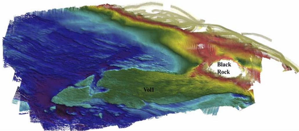
**Figure 4** High-resolution multibeam bathymetric map of the area to the west of Black Rock in Minas Passage, produced by Seaforth Geosurveys Inc. This data formed the basis for a variety of seabed maps on backscatter, slope and relief.
