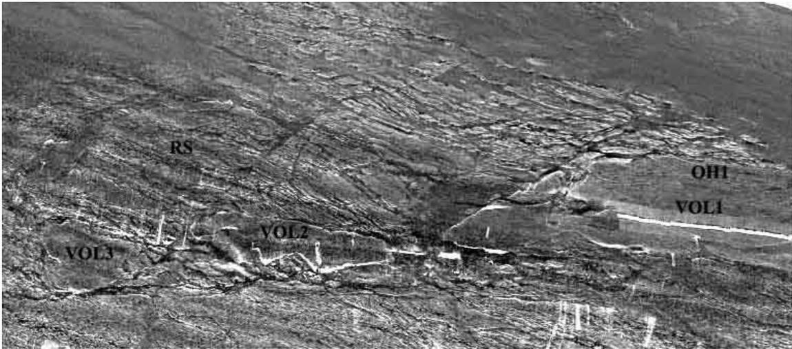
**Figure 15** A regional backscatter image of the sites NSPI/OHI and RS showing that they occur over a very hard seabed of gravel and bedrock. Volcanic ridge segments 1 -3 are identified for reference.
