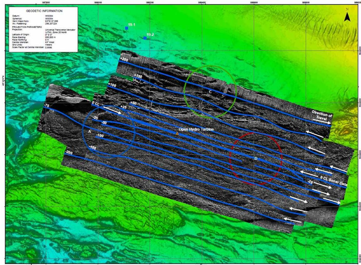
**Figure 7** A sidescan sonar mosaic produced from data collected during the monitoring survey. It is superimposed over the multibeam bathymetry (Background). The location of sites A, C, D and NSPI/OH1 are shown. Direction of travel of the sidescan tow fish is shown by arrows.
