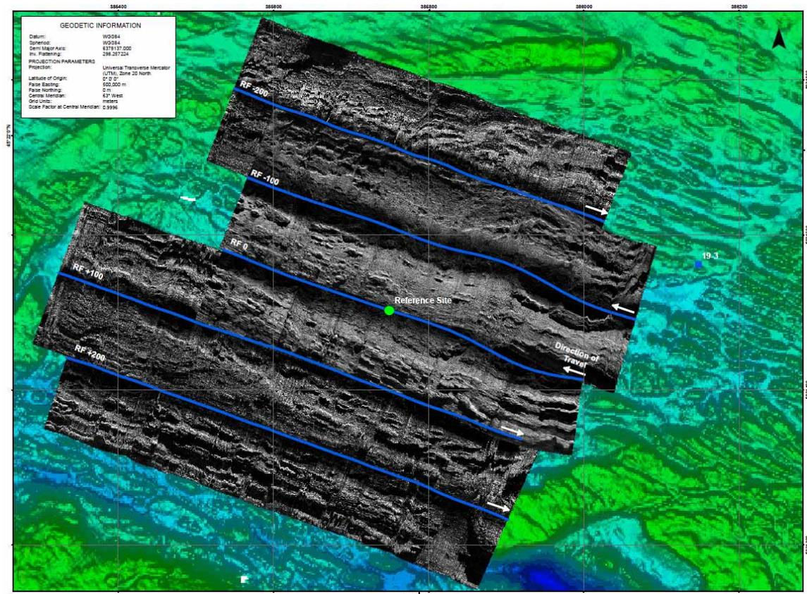
**Figure 9** A sidescan sonar mosaic from the Reference Site overlying multibeam bathymetry. The Reference Site occurs in the centre of the mosaic (green dot). Survey lines and direction of travel are indicated.
