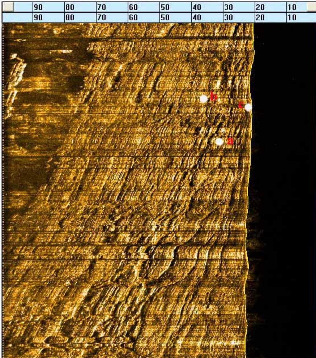
**Figure 26** A sidescan sonogram from the site of NSPI/OH1 collected in 2008. It has been compared with the sonograms collected for the monitoring survey to detect change. However, the quality of the first survey data was less because of excessive fish motion due to strong currents and turbulence that was not present during the monitoring survey. The locations of the three feet of the gravity structure are indicated.
