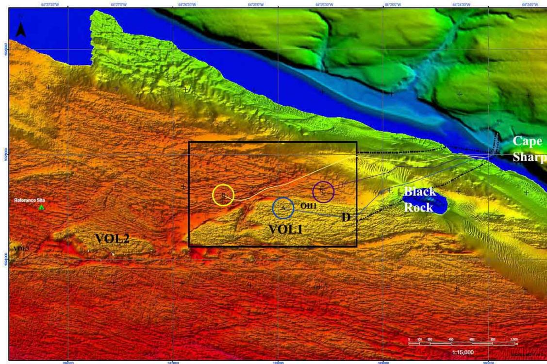
**Figure 3** Multibeam bathymetric shaded-relief image of Minas Passage from data collected by the Geological Survey of Canada and the Canadian Hydrographic Service. Superimposed on the map is the Crown Lease Area (black box), the three original test berths, the new berth D, the location of NSPI/OH1, the Reference Site, and the three volcanic platforms of the region.
