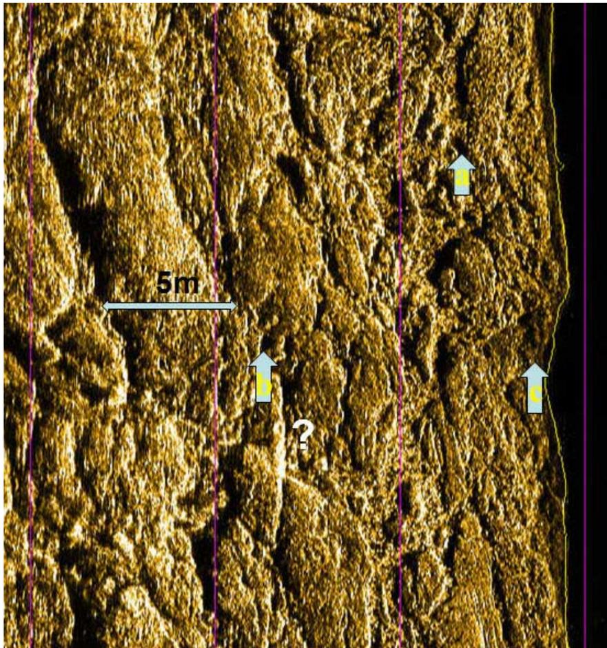
**Figure 25** A sidescan sonogram of the site of NSPI/OH1 showing the position of the feet on the seabed. Arrows are used to indicate the locations and not obscure the actual positions. Note the linear unusual feature near the foot b noted with ?.
