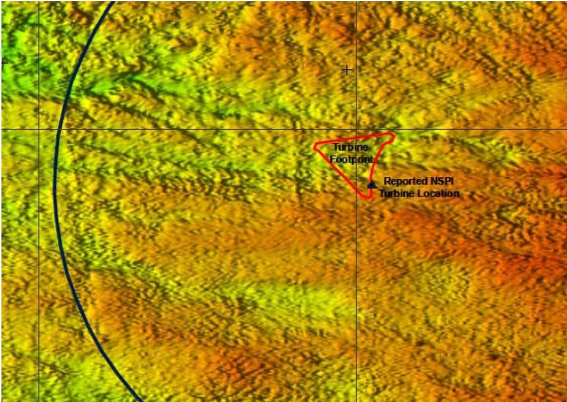
**Figure 24** A high resolution multibeam bathymetric image showing the location of the NSPI/OH1 site on the seabed and the relief of the bottom. From this image the exact location and water depths of the position of the feet can be determined.
