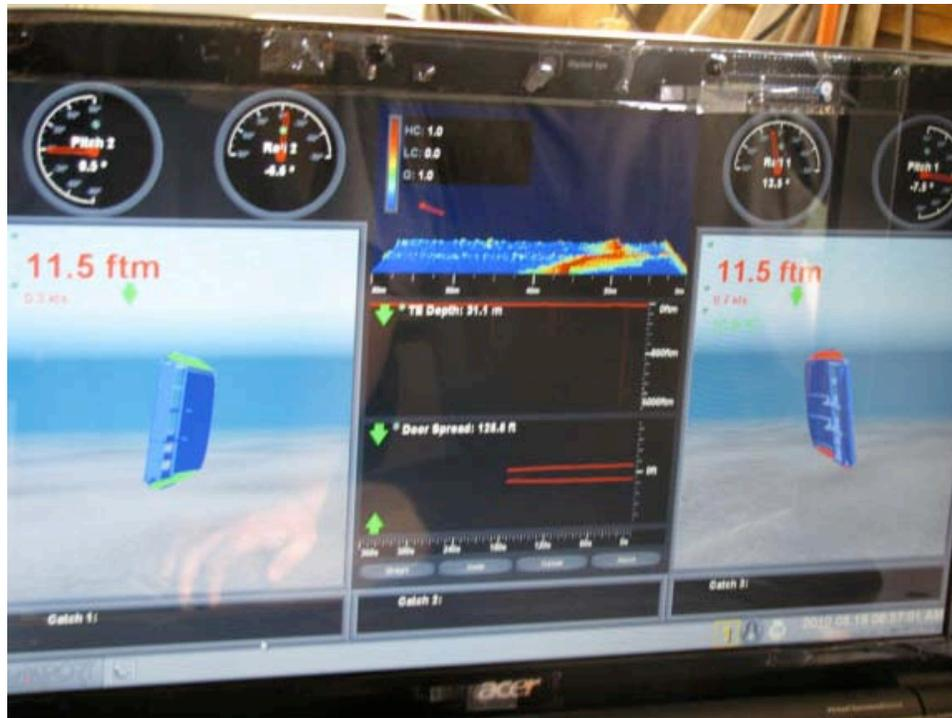
**Photo 2-3: Marport Trawl Sensor Monitoring Display**
