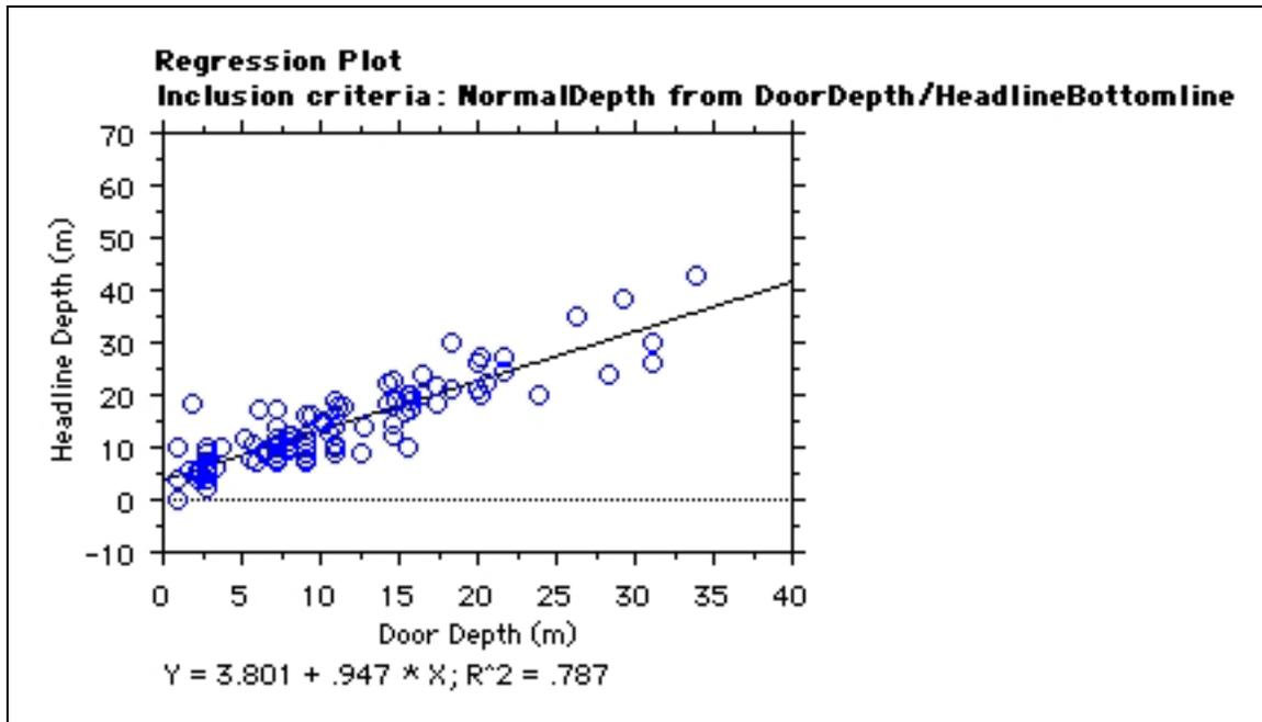
**Figure 2-3: Linear Relationship Between Headline Depth and Door Depth**
