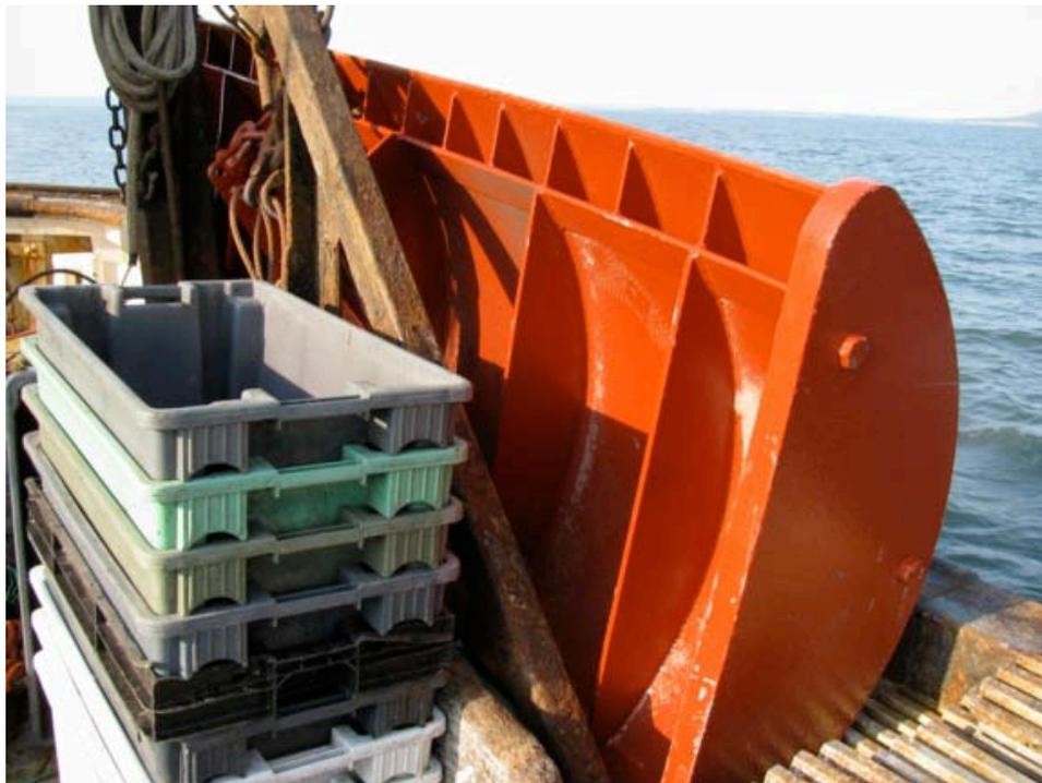
**Photo 2-2: Trawl Door for the Midwater Trawl used on the Carmelle #2**
