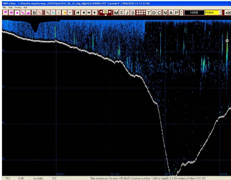
**Figure 3-1: An Echogram Showing Blue Haze (left) and Typical Targets (right)**
