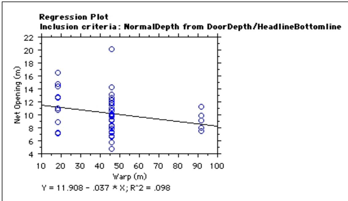
**Figure 2-4: Relationship Between Warp Length and Net Opening**
