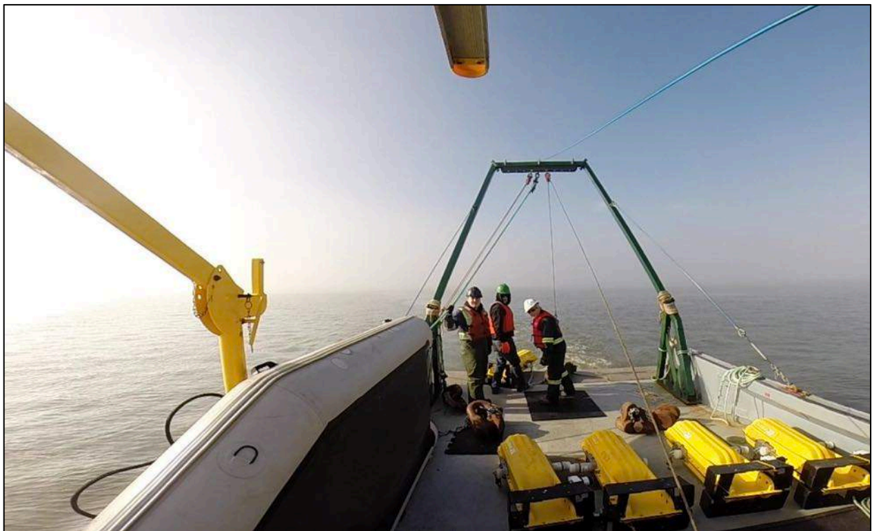
Figure 2: FORCE ocean technologist and crew of the Nova Endeavor (of Huntley's Sub-Aqua Construction from Kentville, Nova Scotia) prepare to deploy C-PODs as part of FORCE's marine mammal monitoring program.
