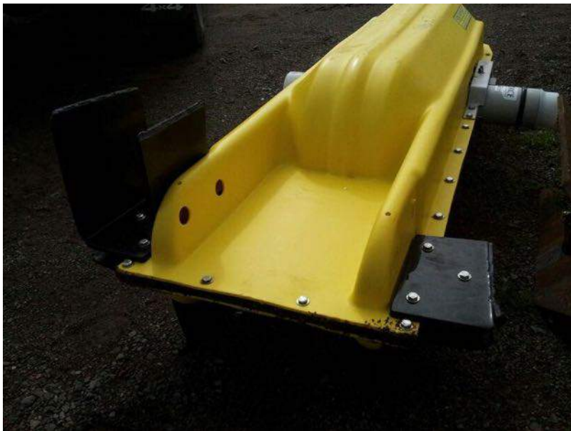
Figure 4: A SUBS package, which housed a C-POD and fish tag receiver, recovered in Diligent River lost its rudder.
