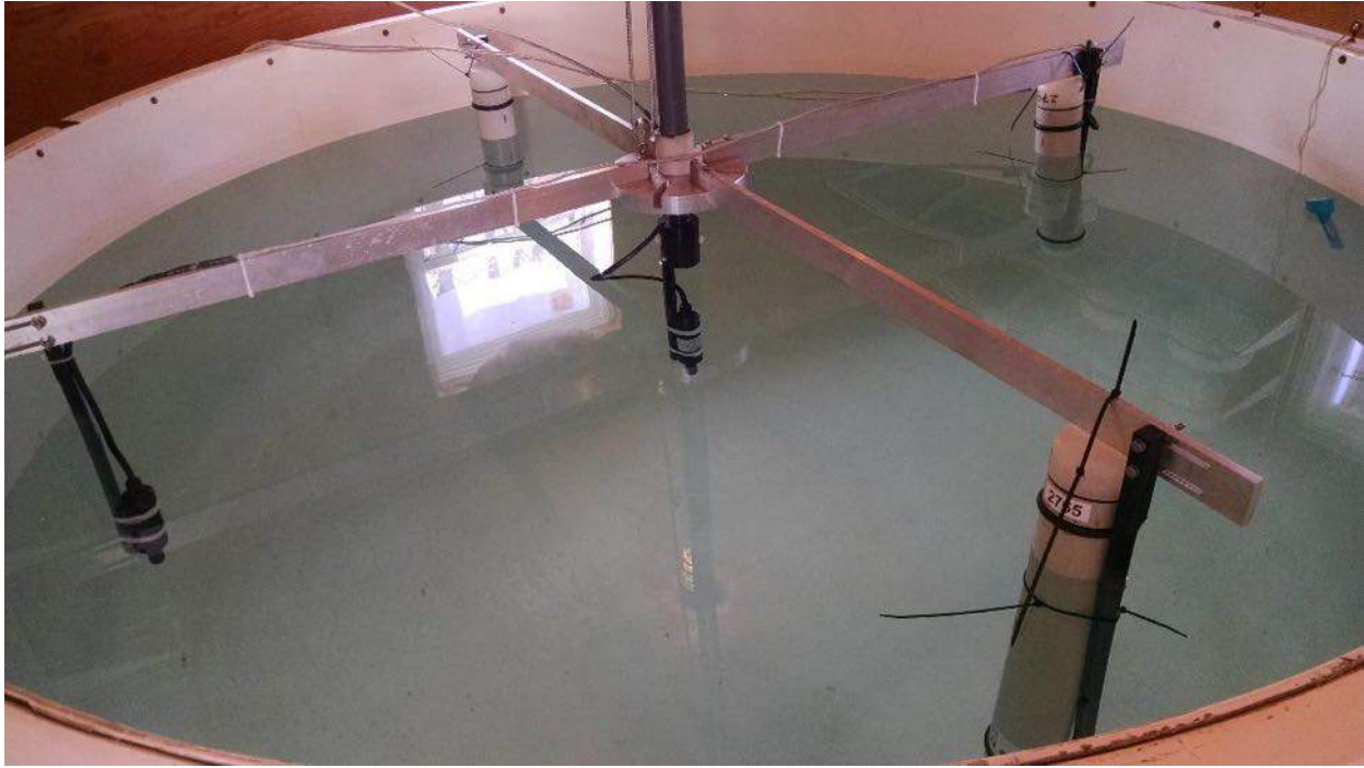
Figure 4. Experimental setup with the icTalk in the center of the tank, 3 C-PODs around the periphery and an icListen reference hydrophone, also at the periphery.
