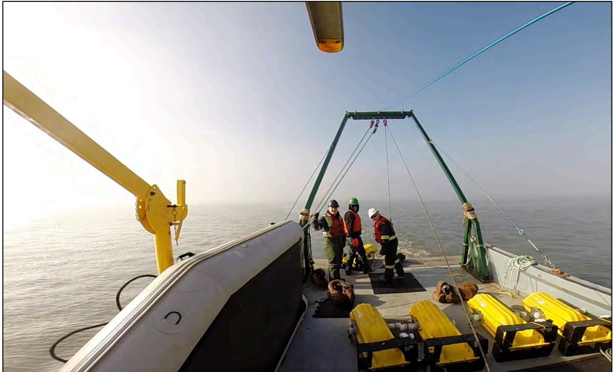
Figure 3: FORCE ocean technologists and crew of the Nova Endeavor (of Huntley's Sub-Aqua Construction from Kentville, Nova Scotia) prepare to deploy C-PODs as part of FORCE's marine mammal monitoring program.
