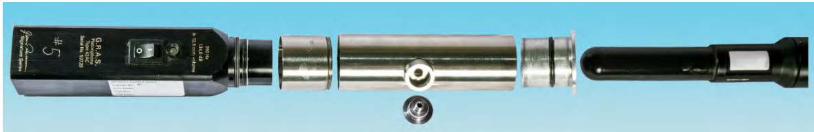
Figure 30. Split view of a G.R.A.S. 42AC pistonphone calibrator with an M36 hydrophone Manufacturers' calibrations were used for the icListen data.
