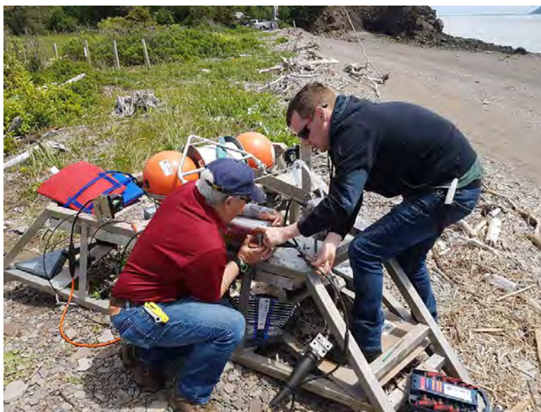
Figure 10: FORCE personnel work on the FAST-2 sensor platform in mid-June, connecting a multibeam imaging sonar camera to a multiplexer, which collects and transmits data to shore via optical fibres.
