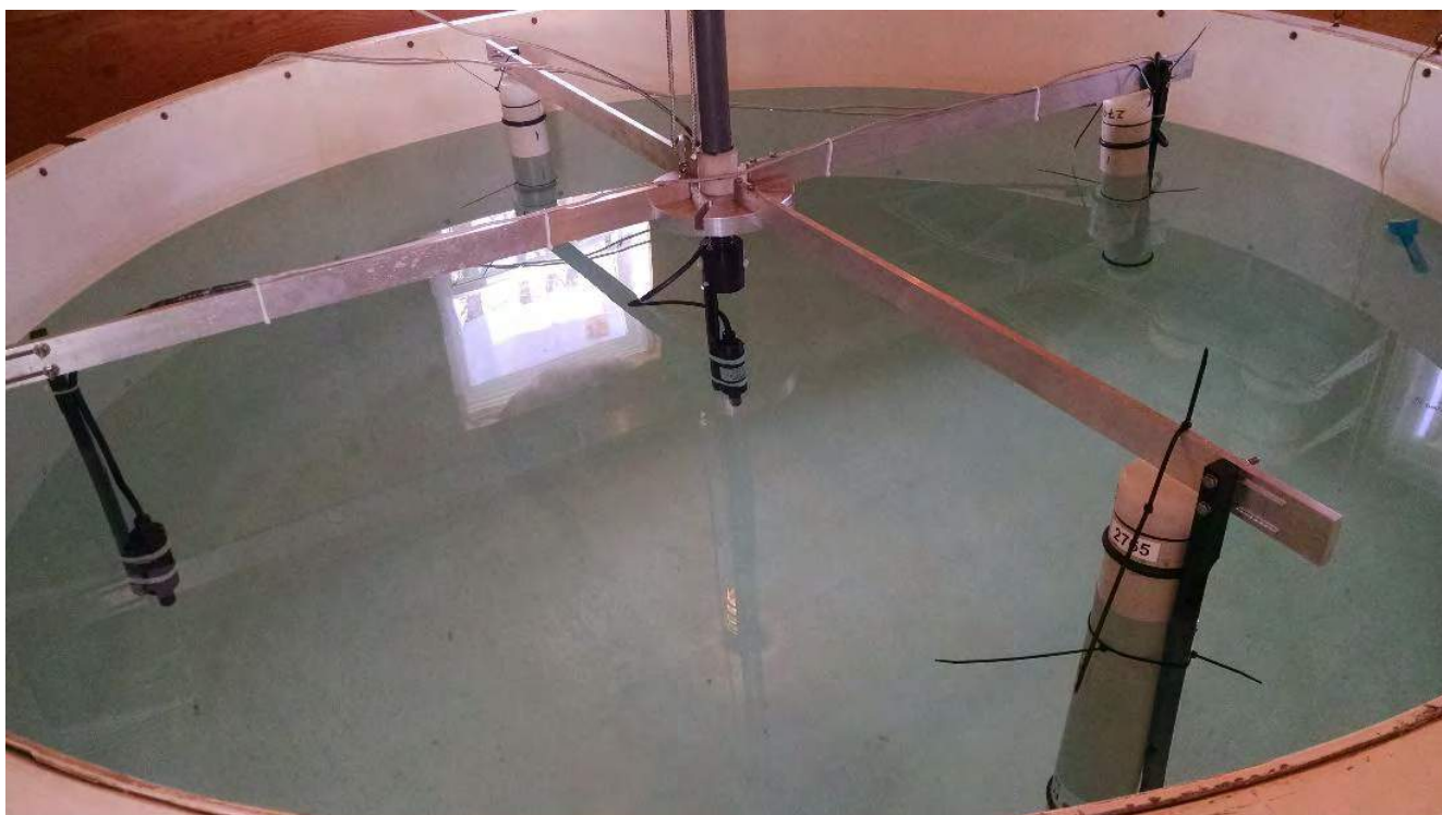
Figure 2. Experimental setup with the Ocean Sonics icTalk projector in the center of the tank, 3 C-PODs around the periphery and an Ocean Sonics icListen reference hydrophone, also at the periphery.
