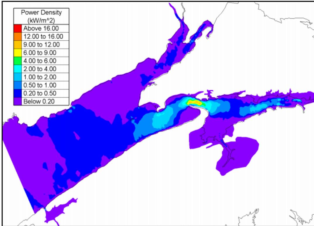
**Figure 4.** Minas Passage power density in kW/m<sup>2</sup> (Cornett, 2006).
