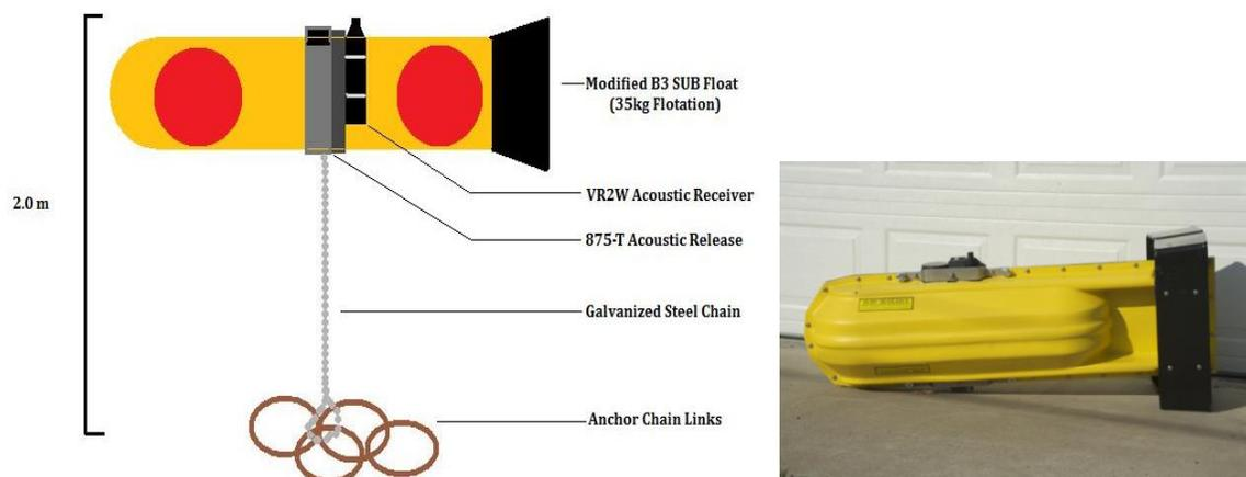
**Figure 2.8.** Left: Diagram indicating internal orientation of the VR2w Receiver and Benthos Teledyne acoustic release (not to scale, from Stokesbury et al., 2012). Right: photo of SUB flotation package with instrument package installed.
