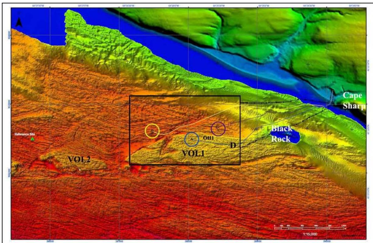
**Figure 4. Multibeam bathymetric map of the FORCE test area and surrounds in Minas Passage, Bay of Fundy (Source: GSC, in Fader 2011), showing volcanic platforms (VOL), gravel waves, troughs, and various bedforms. Black Rock is located east of the FORCE site.**
