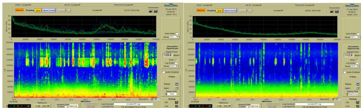
**Figure 33. One minute LUCY screenshots with a high number of click detection events. Left, both the icListenHF and C-POD recorded a DPM. Right, the CPOD did not record a DPM during this minute which shows numerous faint clicks (i.e. clicks were beyond the detection range of C-PODs but within range of the icListenHF).**
