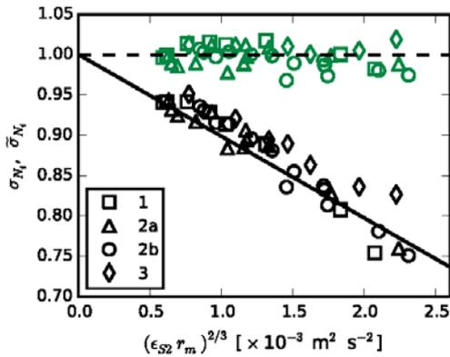
**Figure 4.** Normalized Doppler noise standard deviations for all four sites. The plotted values are averages among the four ADCP beams, where the black and green markers correspond to the uncorrected and corrected values, respectively. (from McMillan and Hay, 2017).
