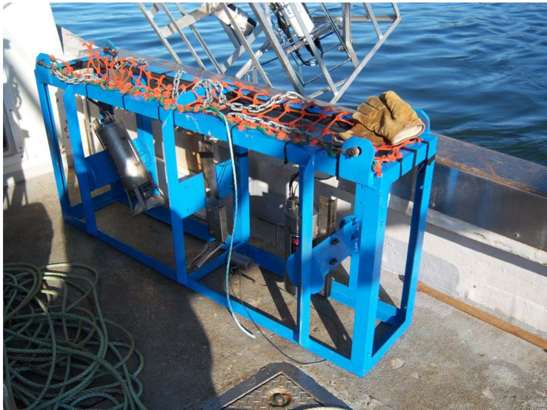
Figure 2. Benthos deep sea camera and frame.
