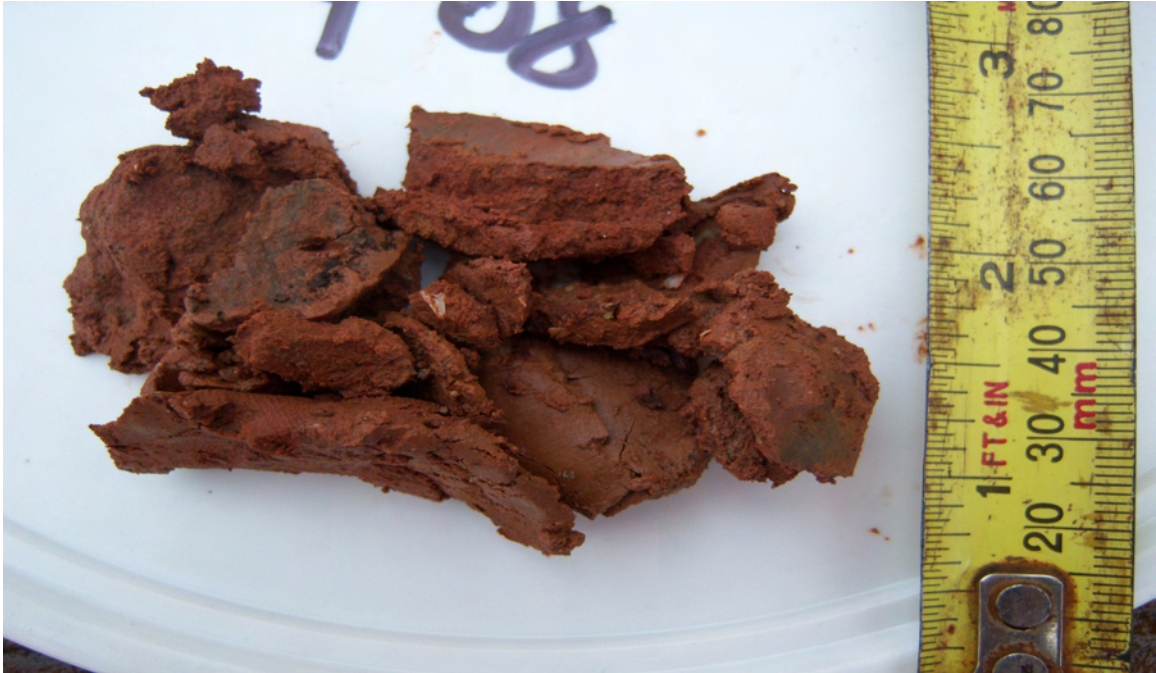
Figure 16. Photograph of a sample of stiff red mud collected by a rock dredge that penetrated the gravel lag surface in the northern area of Minas Passage. The material is similar to cored glaciomarine sediments in other areas of the inner Bay of Fundy that were deposited approximately 13 000 years ago during the retreat of the glaciers from the region. This material may underlie other areas of flat gravel lag in Minas Passage.
