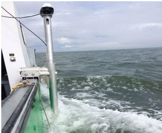
Mobile surveys use a scientific echosounder, the Simrad EK80, mounted on a vessel
