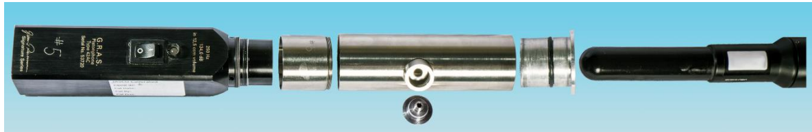
Figure A-7. Split view of a G.R.A.S. 42AC pistonphone calibrator with an M36 hydrophone Manufacturers' calibrations were used for the icListen data.
