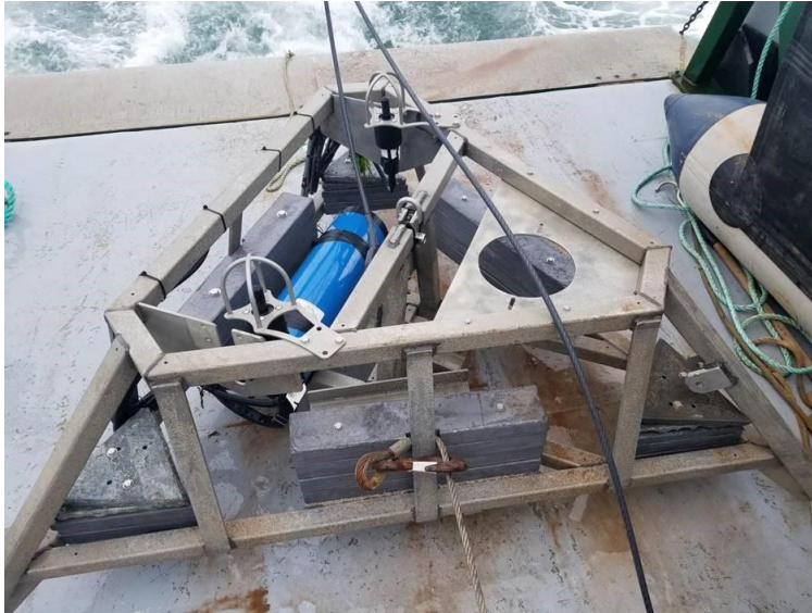
Figure A-2. FAST platform with two icListen hydrophones.
