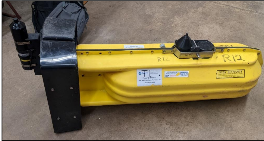
Figure 6: New positioning of acoustic receivers and release mechanism on a SUB package.
