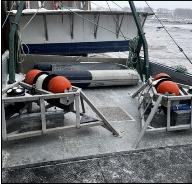
Figure 2: Two Nortek Signature 500 autonomous ADCP's fitted in aluminum frames during deployment at the FORCE tidal demonstration area.
