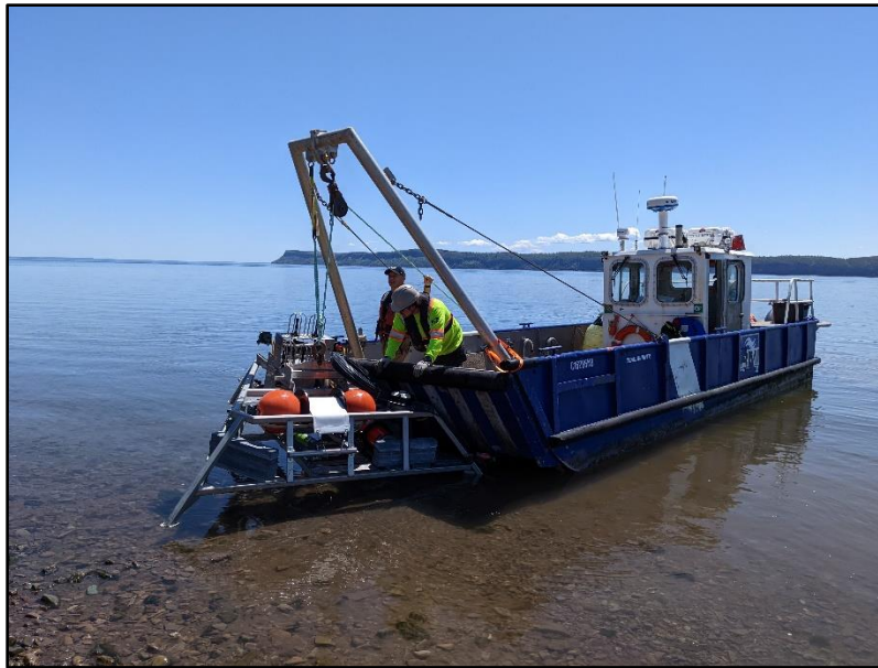
Figure 8: The cabled subsea platform developed for the VITALITY project just prior to deployment at the FORCE test site.
