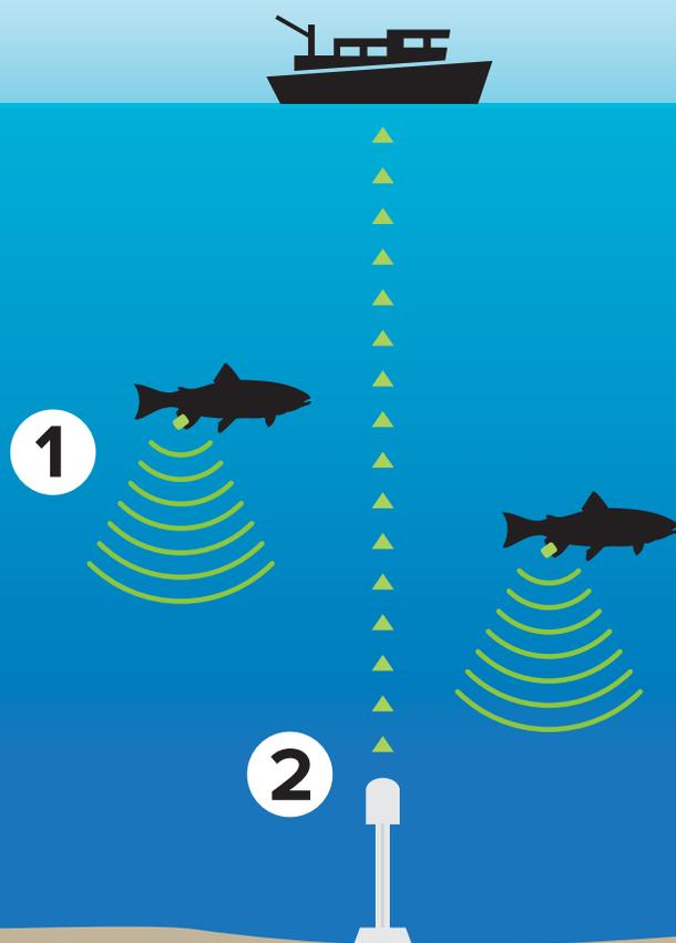
Acoustic tracking is the basis of the fish atlas: tagged fish (1) transmit a signal captured by a network of 12 acoustic receivers (2) which allow us to learn more about their movement in the Minas Passage.
