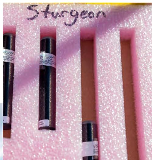
**Above:** Acoustic tags come in different formats and can last up to a decade. Most RAP tags are commonly used frequencies of either 69 kHz or 180 kHz. The choice is mostly dependent on fish size (smaller fish get smaller tags), receiver type and placement.
