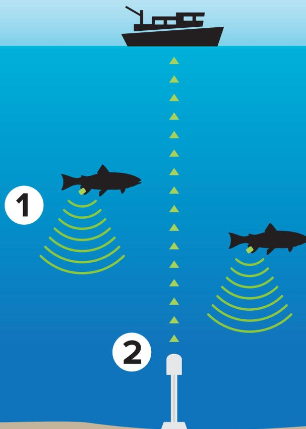
Fish tracking is the basis of the RAP biological data set: tagged fish (1) transmit a signal captured by acoustic receivers (2) which are then recovered to download data and confirm encounter rate model predictions (also see page 6).
