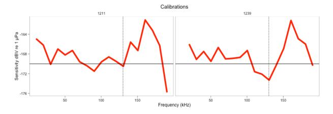
Figure 3.1. Calibration results for icListenHF 1211 and 1239 fitted with HDPE guards. Horizontal bar is a reference at -170 dBV re 1uPa. Vertical dashed line (130 kHz) is within the frequency that harbour porpoises use for echolocation.
