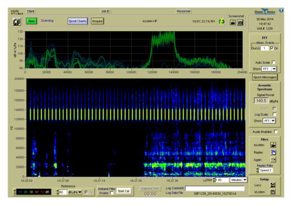
*Figure 3.4 IcListen spectrograms from tank test trials.* **Top:** *without acoustic foam.* **Bottom:** <sup>1</sup>/<sub>2</sub> *inch thick, 20 ppi acoustic foam. The tank test trial commenced half way through the minute.*
