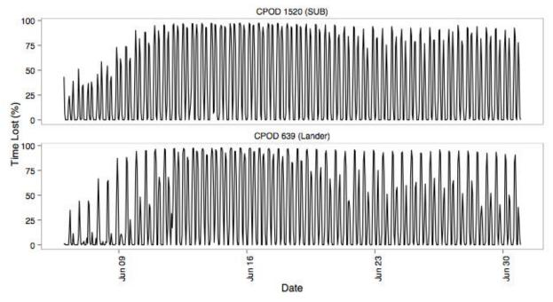
Figure 4.4. C-POD percent lost time plots. **Top:** SUB Buoy mounted C-POD 1520; **Bottom**: platform mounted C-POD 639. The series of peaks represent the sequence of flood and ebb tides during June 2014 with flood tides showing greater % lost time compared to ebb tides. A spring-neap pattern is also evident; a full moon occurred on 13 June 2014.
