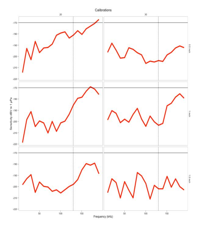
Figure 3.3. Calibration results for icListenHF 1239 for various shroud setups. Horizontal bar is a reference at -170 dBV re 1uPa. Vertical dashed line (130 kHz) is within the frequency that porpoises use for echolocation. Rows represent various acoustic foam thicknesses tested and columns represented pore density (20 ppi and 30 ppi).
