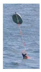
*Figure 4.7. Spar buoy with GPS and radar deflector drifting over the instrument platform (lander). IcTalk speaker unit is drifting 2 m below surface.*
