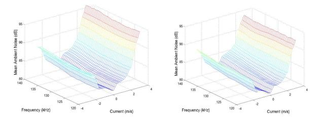
*Figure 4.10. icListenHF hydrophone measures of mean ambient noise (dB) at 120-140 kHz, as a function of current speed (m/s), at location W1 during 6 June - 11 June 2014. Left: hydrophone 1211 without a foam shroud; Right: hydrophone 1239 with*  $\frac{1}{2}$  *inch, 20 ppi acoustic foam shroud.*
