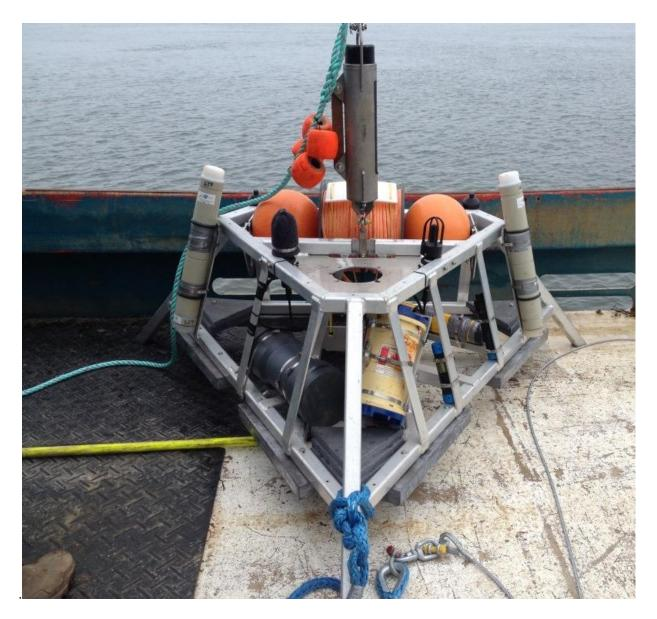
Figure 4.2. Image of instrument platform ready for deployment. Note the 2 C-PODs in the far corners and the shrouded and non-shrouded icListenHF hydrophones (black sensors) located above their battery packs. The instrument hanging vertically above the frame is the Teledyne Benthos 866-a acoustic release.
