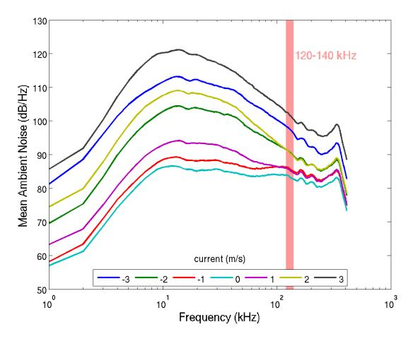
Figure 4.9. icListenHF 1239 hydrophone measures of ambient noise (dB/Hz)in Minas Passage, at FORCE monitoring location W1 during 6 June – 2 July 2014, as a function of frequency (kHz) for a range of current speeds (+/- 0.1 m/s) on the ebb (-) and flood (+) tides. The hydrophone was shrouded (20 ppi,  $\frac{1}{2}$  inch foam) and housed on the bottom moored instrument platform. Note that harbour porpoise echolocation click train frequencies are in the range of 120-140 kHz.
