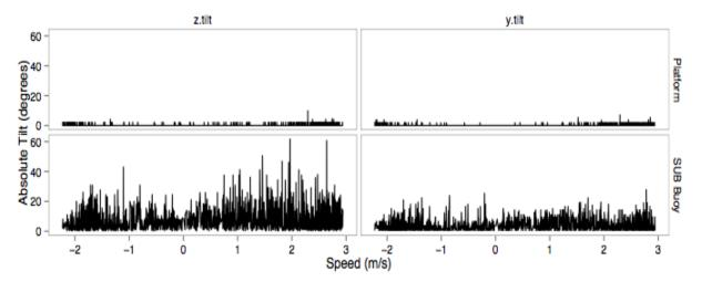
Figure 4.5. Tilt plots comparing pitch (z.tilt) and roll (y.tilt) with depth-averaged current speed (m/s) on the ebb (-) and flood (+) tides for the instrument platform and a SUB buoy located at station location W1.
