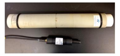
Figure 1.1 Hydrophone images. Top: C-POD (Chelonia Ltd). Bottom: icListenHF (Ocean Sonics Ltd).
