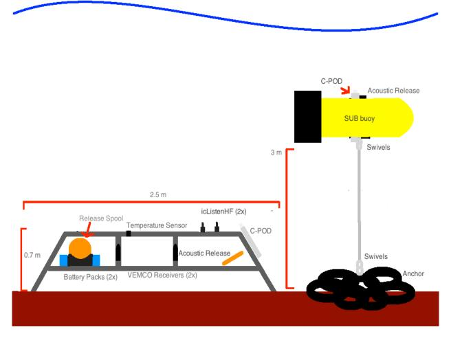
Figure 4.1. Mooring designs. Left: Instrument platform housing two icListenHF hydrophones with battery packs, a C-POD, and an acoustic release, plus other sensors (temperature, VEMCO receivers). Right: SUB buoy housing an acoustic release and a C-POD, and attached to anchor weight (about 200 kg) with a 3 m long riser chain.
