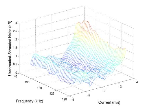
Figure 4.11. The difference in mean ambient noise (dB) between shrouded and unshrouded icListenHF hydrophones in Figure 4.10. Note that the difference is low overall (mostly <1 dB) and greatest at depth-averaged speeds >3 m/s on the flood tide.
