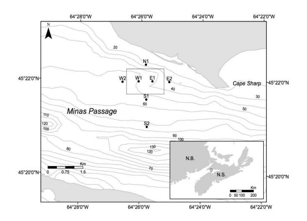
Figure 2.1. Bathymetric map of study location in Minas Passage and multi-year (2010-2014) hydrophone stations at and near the FORCE test site. FORCE dimensions (rectangle) are 1.0 km x 1.6 km. Stations E2, S2 and N1 not included in the current study.
