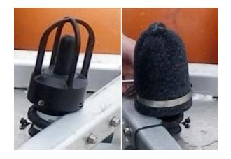
Figure 3.2. IcListenHF hydrophone tip with custom made HDPE guard (left) and with a  $\frac{1}{2}$  inch 20 ppi foam cover secured over the guard (right).
