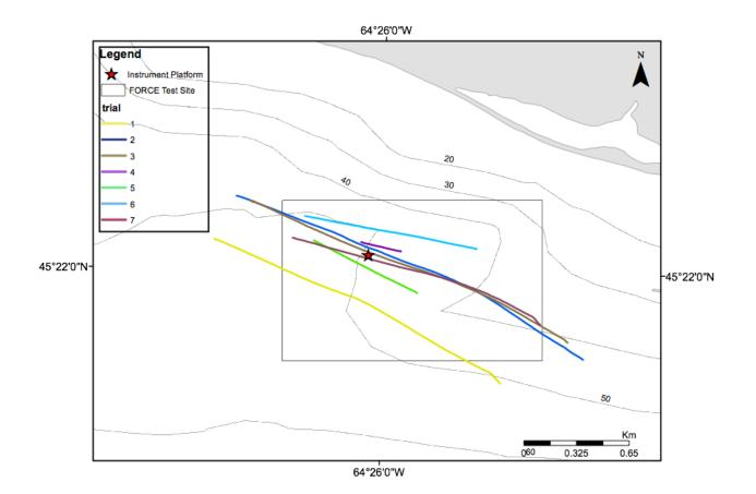
Figure 4.6. icTalk speaker tracks through the FORCE site and over the instrument platform (red star).
