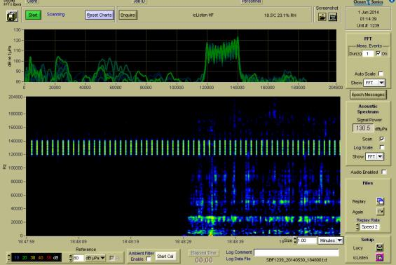
*Figure 3.5. IcListen spectrograms from tank test trials.* **Top:** *without acoustic foam.* **Bottom:** 1 *inch thick,* 20 *ppi acoustic foam.* The tank test trial commenced half way through the minute.
