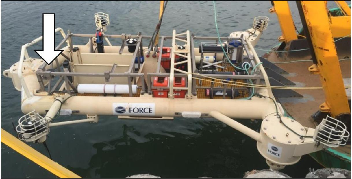
Figure 1. FAST-1 sensor platform developed by FORCE and deployed at the FORCE test site from 8 December 2015 to 5 January 2016. White arrow indicates location of AZFP transducer. Photo credit: Tyler Boucher.
