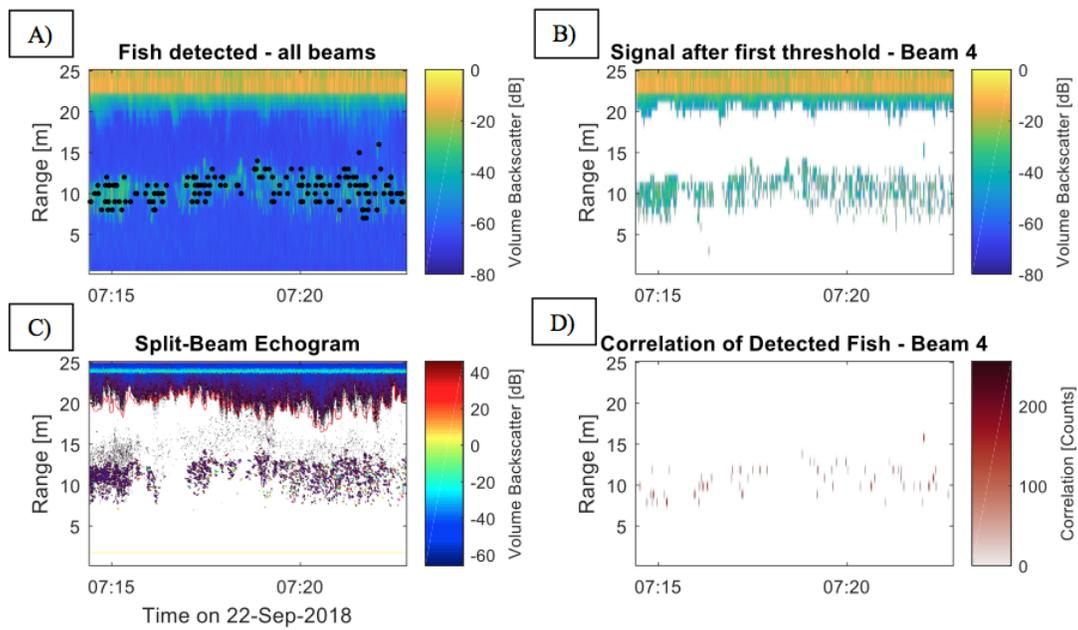
Figure 11: A) A volume backscatter echogram from the ADCP of a fish school, with the identified fish targets (.) from all four beams. B) The remaining data after the backscatter threshold is applied. C) The corresponding split-beam echosounder signal. D) Return signals that met or surpassed the intensity and correlation thresholds. Figure from *Dunn* (2019).
