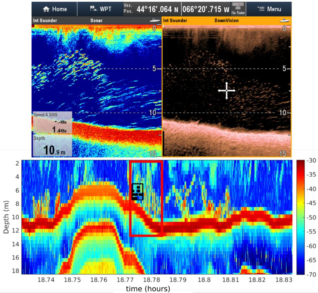
Figure 22: (Top) Fish school observed using the Puffin’s Raymarine echosounder in Grand Passage, August 26, 2019. (Bottom) Backscatter intensity data, in dB re  $1 \text{ m}^{-1}$ , from beam 1 of the Nortek Signature500 ADCP deployed aboard the Puffin. The red box corresponds to the time and space intervals shown in the Raymarine echogram. Fish velocity estimates were computed using a subset of the fish school, shown by the black box. Detected fish are indicated by black dots.
