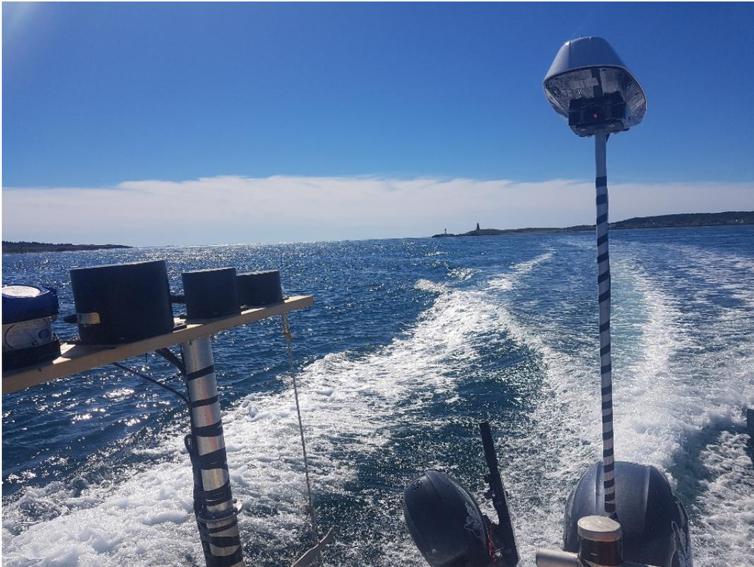
Figure 3: Vessel-mount configuration aboard the RV Puffin in Grand Passage. The four instruments on the pole mount (left of image) from left to right are the 600 kHz RDI ADCP and the 38 kHz, 120 kHz, and 200 kHz BioSonic DTX transducer heads. The post on the right is a GPS receiver.
