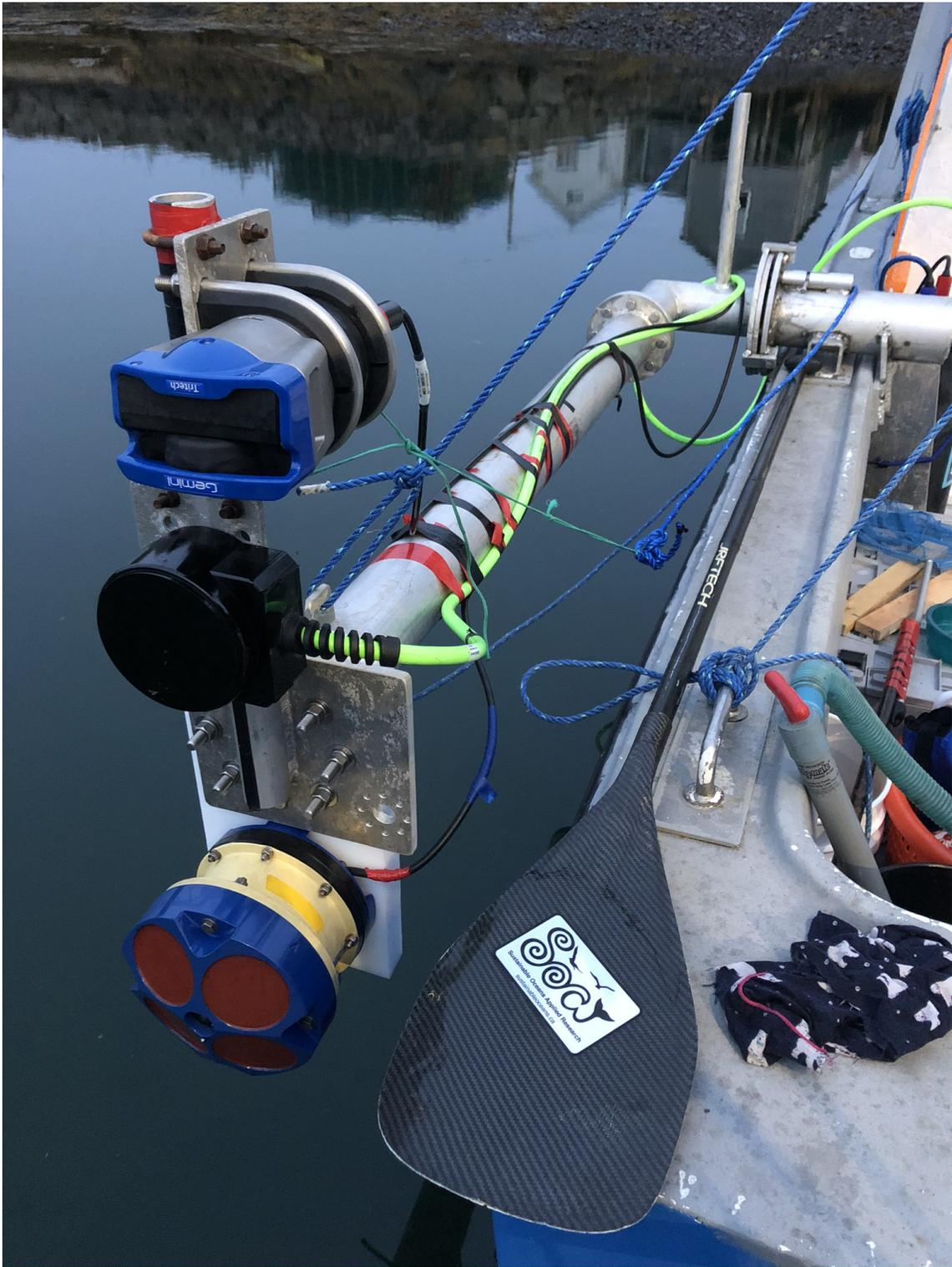
Figure 6: Instrument mounting pole in the undeployed position aboard the RV Grand Adventure. The 600 kHz RDI Workhorse Sentinel ADCP and 120 kHz BioSonics DTX split-beam echosounder are the bottom and middle instruments, respectively. The third instrument (highest in the photo) is a Tritech Gemini multibeam sonar which was not used for the purposes of this report.
