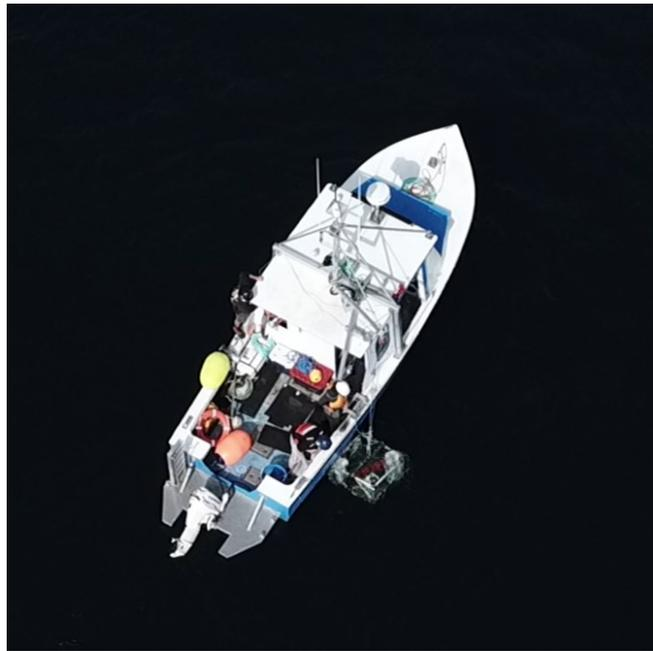
Fig. 2.6.4: Deployment of the receiver using the hoist
