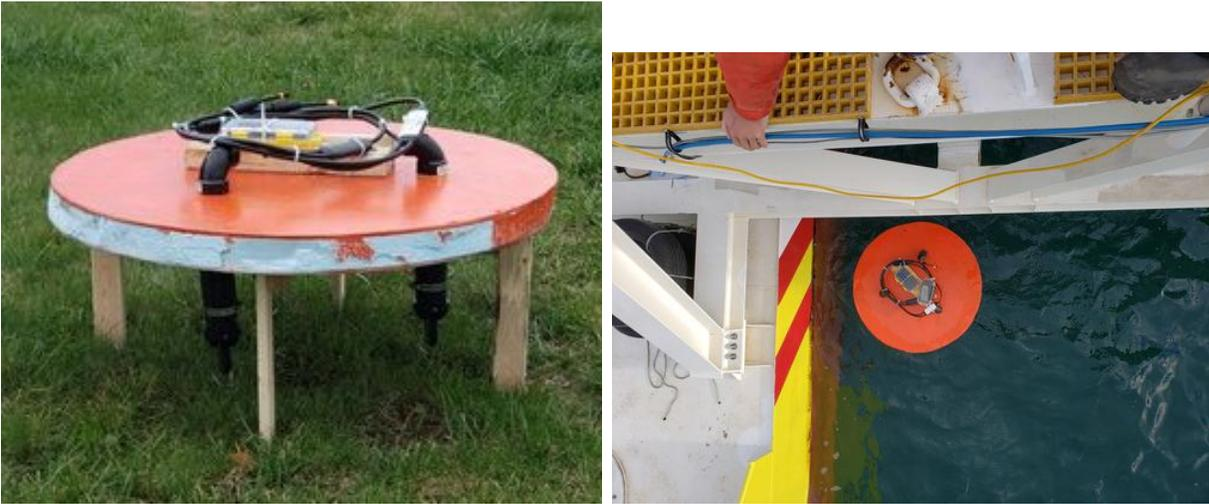
Figure 36: LEFT: Pad-float hydrophone-array on a wooden stand, showing Smart Cable and GPS/compass above and hydrophones below. RIGHT: Deployed and passing between the hulls of PLAT-I. Photo credit: Mike Adams.
