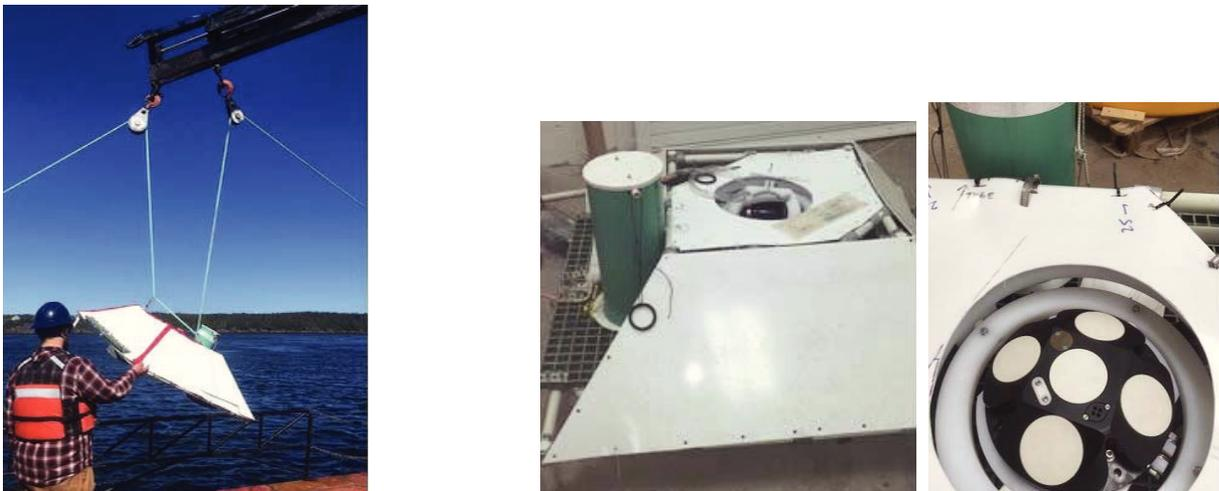
Figure 1: Left panel: The Signature500 being deployed, showing the flow shield skirt (white) and the top part of the tower for the float-line recovery system (green). Middle and right panels: the frame during construction, showing the recovery system tower containing the float and recovery line, the flow shield skirt, and the ADCP in its gimbal mount.
