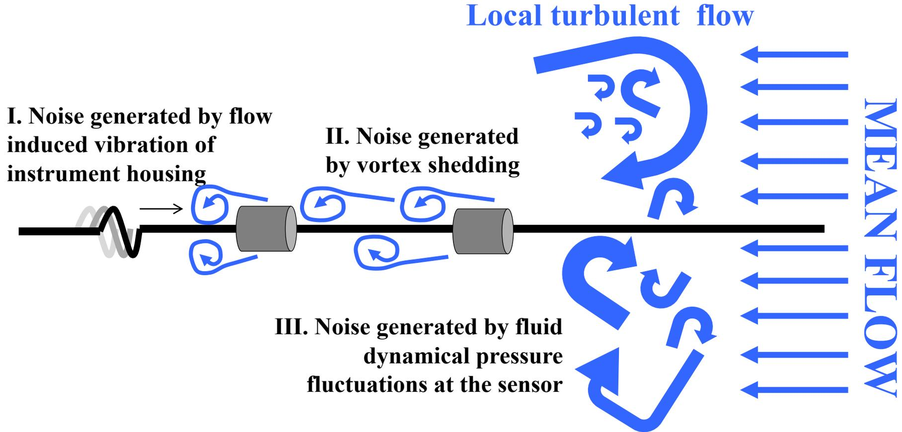
*The sensor provides a spatial average of the noise generated by turbulent flow.*
