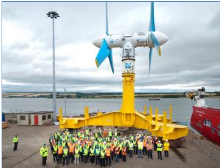
Figure 2.1: Precursor device: Atlantis' 1MW AK1000 turbine, deployed in Scotland, Summer 2010
