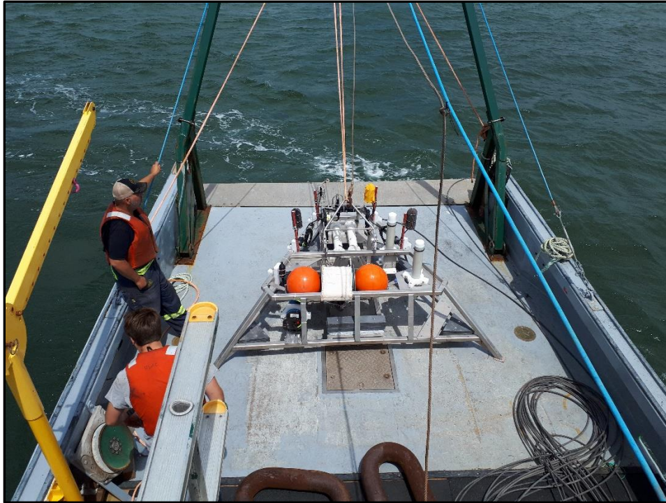
Figure 2: Five PAM devices were mounted on the FAST platform for the comparative PAM study. Photograph depicts the platform on the deck of the Nova Endeavour prior to deployment at the FORCE site.
