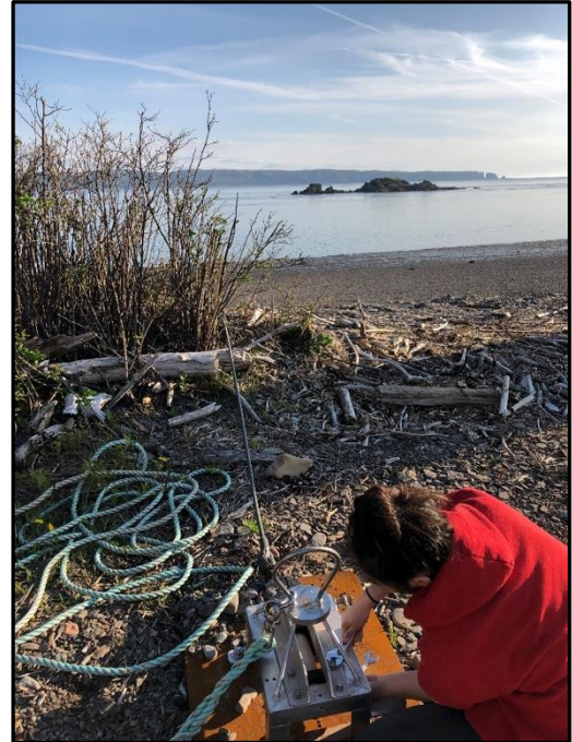
Figure 3: One of FORCE's Ocean Technicians prepares the tide gauge for deployment.
