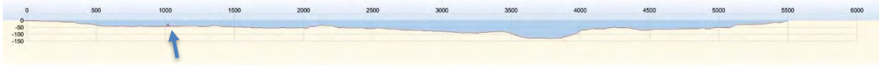
Figure 1: The scale of a single turbine (based on the dimensions of the OpenHydro turbine deployed by CSTV, indicated by the red dot and above the blue arrow) in relation to the cross-sectional area of the Minas Passage. The Passage reaches a width of \sim 5.4 km and a depth of 130 m.
