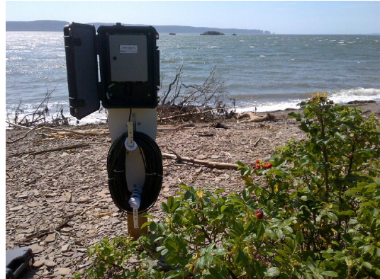
FORCE tide gauge: first device to measure tide level changes in real time.
